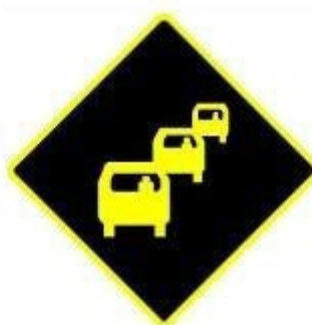
Figure 22 Queue Warning (W163)
