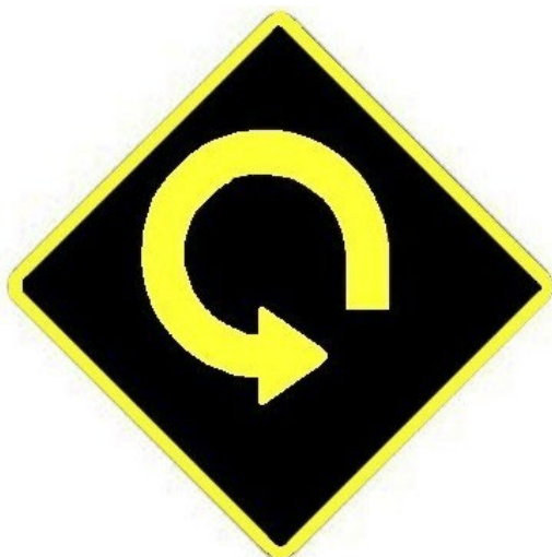
Figure 8 Bend Warning (Left Hand Bend W033)
